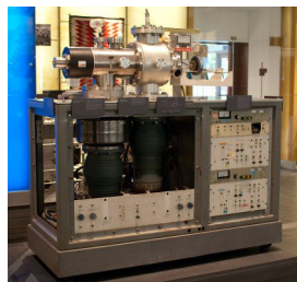
The single quadrupole mass spectrometer and ion source used for Prof. John Fenn's Nobel Prize winning discovery of electrospray ionization.
